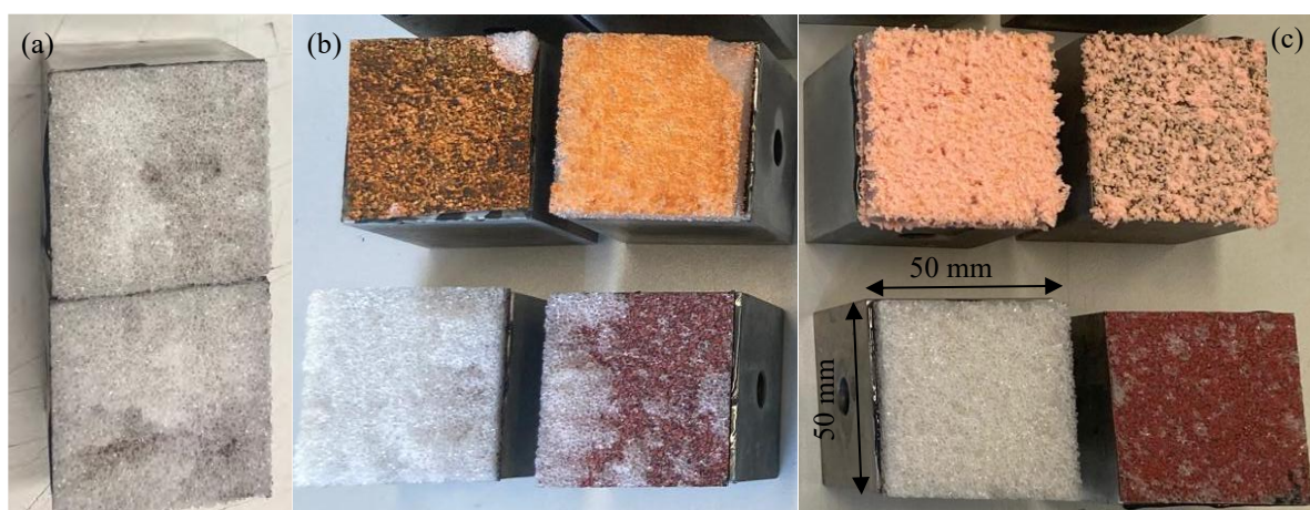
Figure 5 – Flatwise tensile test samples showing (a) a sample without primer with rupture within the foam; (b) samples with 30 gsm P170 primer virgin (bottom) and heat activated (top); (c) samples with 60 gsm P170 primer virgin (bottom) and heat activated (top).
